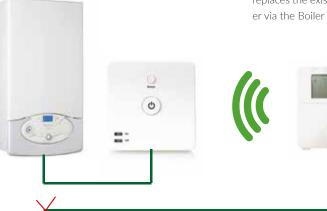
The wireless LightwaveRF Home Thermostat replaces the existing one and controls the boiler via the Boiler Switch
